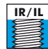
for right- and left hand internal thread for left hand thread modify your NC-program!
